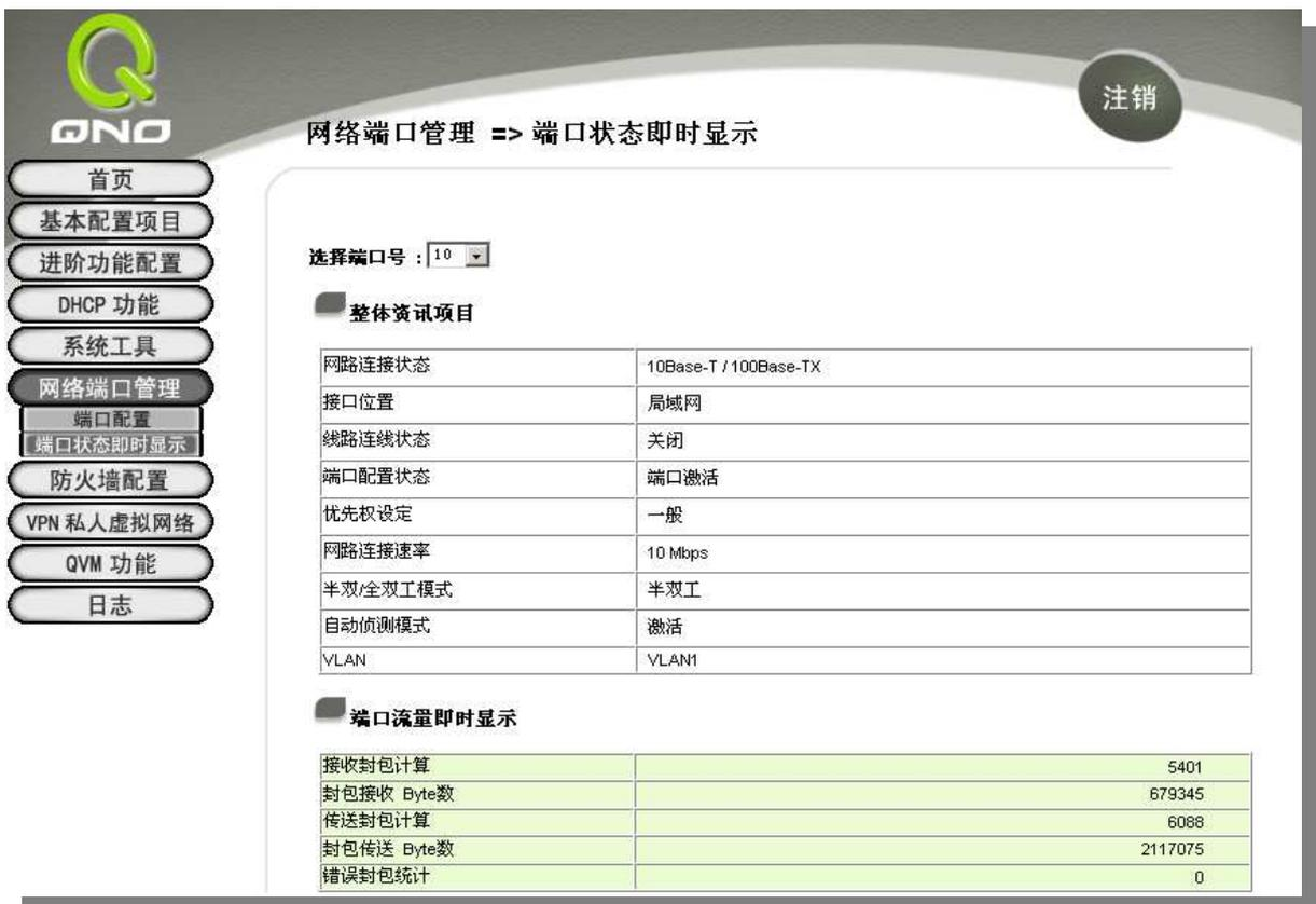
The screenshot shows the QNO web interface for network port management. The left sidebar contains navigation buttons: 首页, 基本配置项目, 进阶功能配置, DHCP 功能, 系统工具, 网络端口管理 (selected), 端口配置, 端口状态即时显示 (selected), 防火墙配置, VPN 私人虚拟网络, QVM 功能, and 日志. The main content area is titled "网络端口管理 => 端口状态即时显示" and includes a "注销" button. A dropdown menu shows "选择端口号 : 10".
