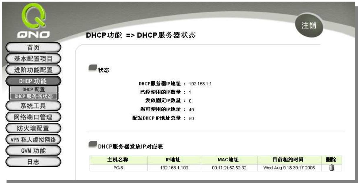
The screenshot shows the DHCP server status page in the QNO web interface. The page title is "DHCP功能 => DHCP服务器状态". On the left is a navigation menu with options like "首页", "基本配置项目", "进阶功能配置", "DHCP 功能", "DHCP 配置", "DHCP 服务器状态", "系统工具", "网络端口管理", "防火墙配置", "VPN 私人虚拟网络", "QVM 功能", and "日志". The main content area shows the following information:
