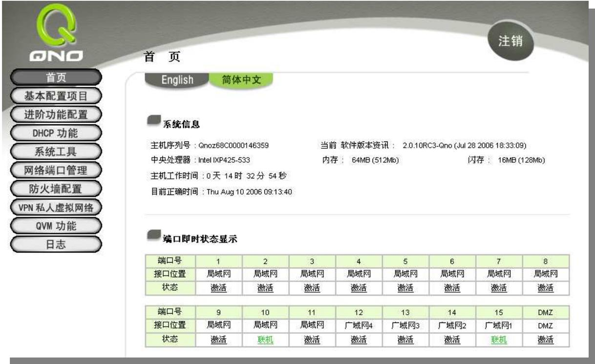
The screenshot shows the 'System Information' page of a QNO router. It includes a sidebar with navigation options like 'Basic Configuration', 'Advanced Configuration', and 'System Tools'. The main content area displays system details and a table of port statuses.
